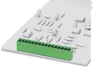
Header, nominal current: 8 A, rated voltage: 160 V, pitch: 3.5 mm, no. of positions: 11, mounting: Soldering
